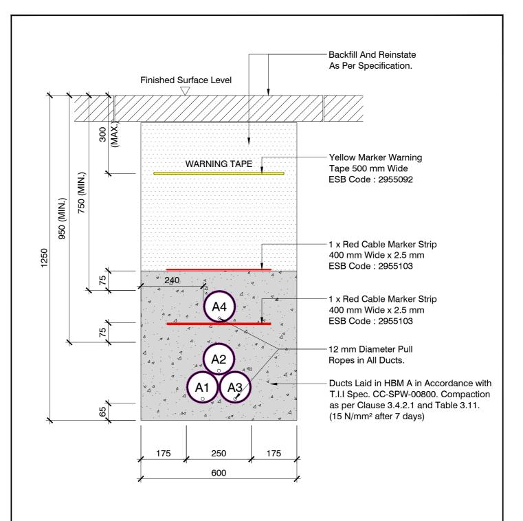
A=125 mm: Outer Diameter HDPE ESB Approved Duct, SDR=17.6
